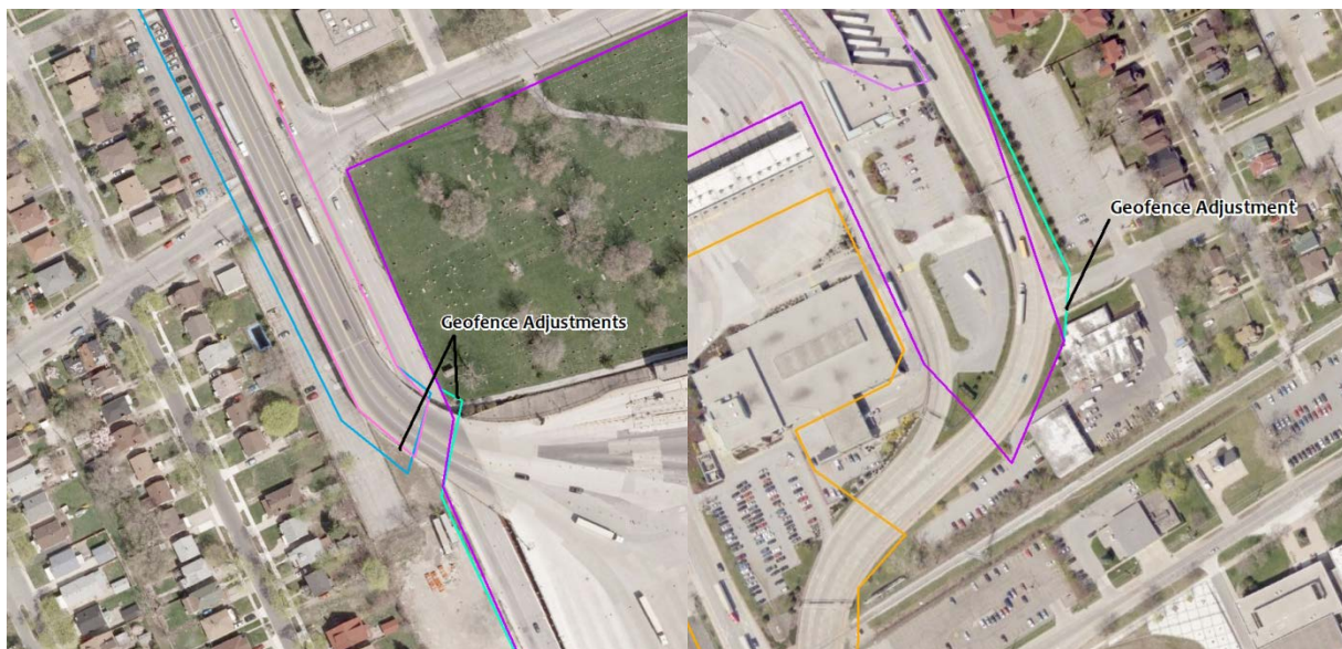
Figure 5-6: Geo-fence adjustments made at the Ambassador Bridge Canada Customs plaza in Windsor, ON. The changes made were minor, and intended to minimize trucks 'jumping' in and out of geo-fences.
